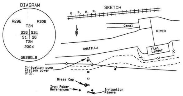
Monument and accessories set: (Procedures and description) I set a 1 3/8" x 30" galvanized iron pipe with an attached 2 3/8" brass cap stamped as shown in the diagram above 54" in the ground.
