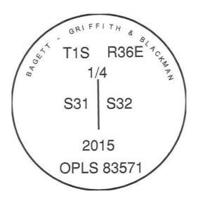
I used a steel tape and magnetic compass in the establishment of the new accessories. I used 16° East declination, the distances are to a 60d spike driven into the right side of the root crown of the bearing trees, spike in left side of the root crown of the Southeast Lodgepole pine bearing tree. A brass washer marked OPLS 83571 is attached to the BT blaze of the new bearing trees.
