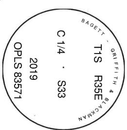
I used a steel tape and magnetic compass in the establishment of the new accessories. I used 13° East declination, the distances are to a 60d spike driven into the side of the root crown of the bearing trees. A brass washer marked OPLS 83571 is attached to the BT blaze of the new bearing trees.
