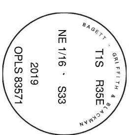
I used a steel tape and magnetic compass in the establishment of the new accessories. I used 13 East declination, the distances are to a 60d spidriven into the side of the root crown of the bearing trees. A brass washer marked OPLS 83573 is attached to the BT blaze of the new bearing trees. the S 83571 spike
