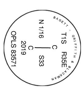
I used a steel tape and magnetic compass in the establishment of the new accessories. I used 1 East declination, the distances and bearings ar to the center of the " $X^{\prime\prime\prime}$ . d 13°
