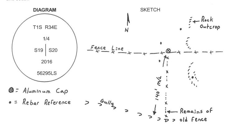
MONUMENT (S) AND ACCESSORIES SET (Procedures and Description) At the position of the original stone I set a 1"x24" iron rebar with a 2" aluminum cap stamped as shown in the diagram above.
