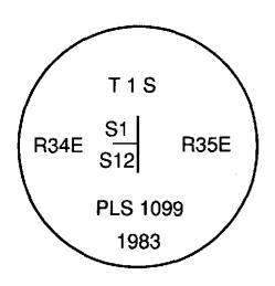
I used a steel tape and magnetic compass in the establishment of the new accessories. I used  $16^\circ$  East declination, the distances are to a 60d spike driven into the right side of the root crown of the new bearing tree. A brass washer marked OPLS 83571 is attached to the BT blaze of the new bearing tree.
