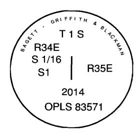
I used a steel tape and magnetic compass in the establishment of the new accessories. I used 16° East declination, the distances are to a 60d spike driven into the right side of the root crown of the new bearing trees. A brass washer marked OPLS 83571 is attached to the BT blaze of the new bearing trees.
