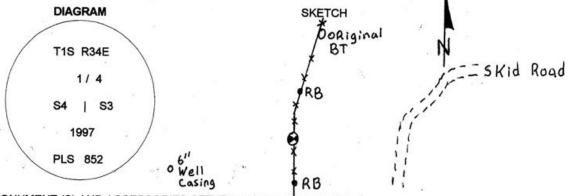
MONUMENT (S) AND ACCESSORIES SET (Procedures and Description) Set a 1 1/4" x 30" Galvanized Iron Pipe with a 2 1/2" brass cap stamped a shown in the diagram above at the position of the rotten post. The cap is 6" above the surface of the ground with a collar of stone.
