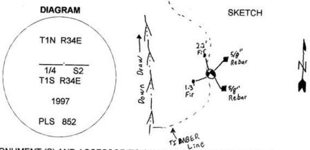
MONUMENT (S) AND ACCESSORIES SET (Procedures and Description) Set a 2 1/2" Brass cap on a 1 1/4"x30" galvanized iron pipe 27" in the ground on the east side of a steep draw at the edge of the timber stamped as shown in the diagram above.
