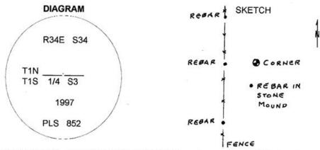
MONUMENT (S) AND ACCESSORIES SET (Procedures and Description) Set a 1 1/4" x 30" Galvanized Iron Pipe with a 2 1/2" brass cap stamped a shown in the diagram above at the position of the surveyed point. The cap is 6" above the surface of the ground with a collar of stone.
