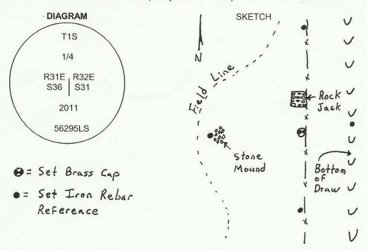
MONUMENT (S) AND ACCESSORIES SET (Procedures and Description) At the position of the found stone I set a 2 3/8" brass cap on a 1 1/2x30" galvanized iron pipe flush with the surface of the ground.
