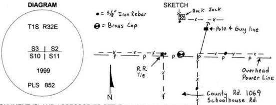
MONUMENT (S) AND ACCESSORIES SET (Procedures and Description) Set a 1 1/4" x 30" Galvanized Iron Pipe with a 2 1/2" brass cap stamped a shown in the diagram above at the position of the stone and post in the county road. Burried the stone and decayed wood along side the cap.
