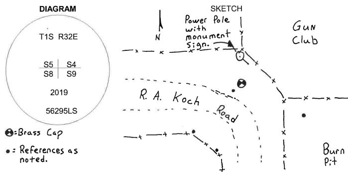
MONUMENT (S) AND ACCESSORIES SET (Procedures and Description) Set a 1 1/4" x 30" Galvanized Iron Pipe with a 2 1/2" brass cap stamped as shown in the diagram
