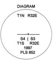
Evidence Found: Found Mr. Perry's stone 18" below surface under an east - west fence line. A 3" iron pipe set by PLS 1333 under survey I-44-B bears S89°52'E, 49.69 feet.
