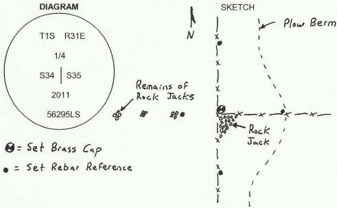
MONUMENT (S) AND ACCESSORIES SET (Procedures and Description) I held the fence intersection and at the corner point I set a 2 3/8" brass cap on a 1 1/2" x 18" galvanized iron pipe 18 inches into the ground to bedrock.
