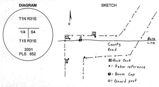
MONUMENT (S) AND ACCESSORIES SET (Procedures and Description) At the point calculated from Staebler's monuments to the south I set a 30" x 1 1/2" G.I.P. with a 2 1/2" brass cap stamped as shown in the diagram above flush with the surface. I set a 5' steel guard post with a County Monument sign attached along side.
