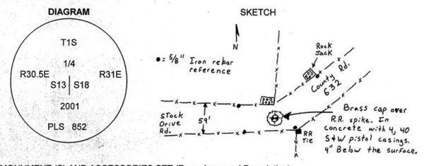
MONUMENT (S) AND ACCESSORIES SET (Procedures and Description) I determined the right of way centerline as midway between the right of way fences and held the intersection of this line with the line of the North - South fence along the township line. At the
