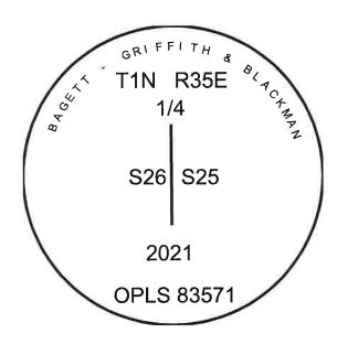
I used a steel tape and magnetic compass in the establishment of the new accessories. I used 14° East declination. Distances are to a 60d spike driven into the right side of the root crown of the bearing trees. Bearings are to a brass washer marked OPLS 83571 is attached to the BT blaze of the new bearing trees.
