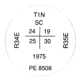
I used a steel tape and magnetic compass in the recovery of the bearing trees and establishment of new trees. I used 16° East magnetic declination and the bearings and distances are to the center of root crown on old bearing trees. Distance is to a 60d spike in the right hand side of the new trees. Bearing is to a brass washer marked OPLS 83571 in the lower BT blaze.
