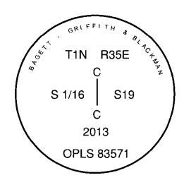
I used a steel tape and magnetic compass in the recovery of the bearing trees. Magnetic declination used was  $16^{\circ}$  East. Bearings are to a brass washer marked OPLS 83571 in the lower BT blaze. Distances are to a 60d spike in the right hand side of the root crown of the bearing trees.
