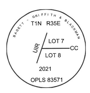
I used a steel tape and magnetic compass in the establishment of the new accessories. I used 14° East declination. Distances are to a 60d spike driven into the right side of the root crown of the bearing trees. Bearings are to a brass washer marked OPLS 83571 is attached to the BT blaze of the new bearing trees.
