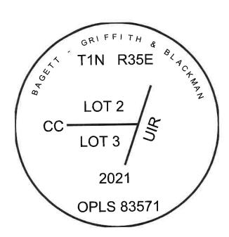
I used a steel tape and magnetic compass in the establishment of the new accessories. I used 14° East declination. Distances are to a 60d spike driven into the right side of the root crown of the bearing trees. Bearings are to a brass washer marked OPLS 83571 in the BT blaze of the new bearing trees.
