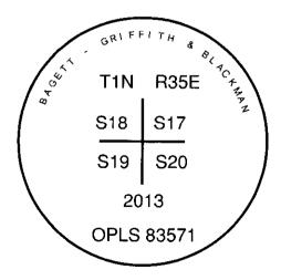
I used an Leica 1200 RTK GPS in the recovery and establishment of the accessories. Measurements are to the center of the caps. Basis of bearing is true geodetic North at the Southwest corner of Section 18, Township 1 North, Range 35 East of the Willamette Meridian as established by GPS observation.
