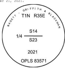
I used a steel tape and magnetic compass in the  $\,$ establishment of the new accessories. I used 14  $^{\circ}$ East declination. Distances are to a 60d spike driven into the right side of the root crown of the bearing trees. Bearings are to a brass washer marked OPLS 83571 in the BT blaze of the new bearing trees.
