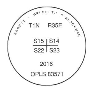
I used a Leica RTK GPS in the establishment of the accessories. Basis of bearing is as per survey for Hancock Forest Management, dated May 2016.
