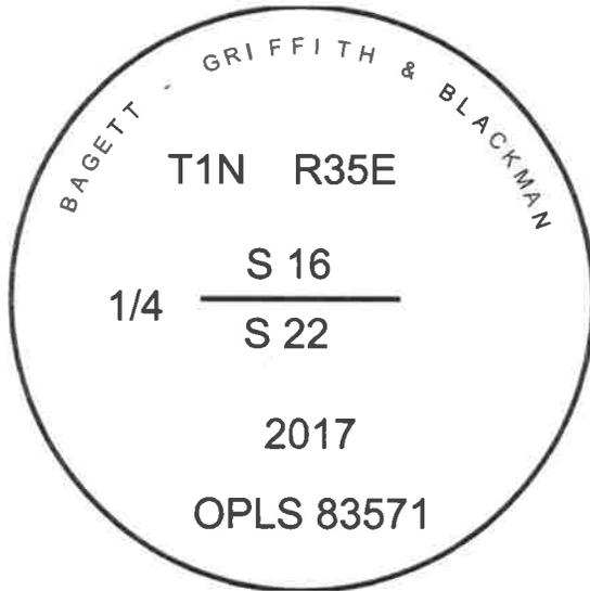
I used an RTK GPS in the establishment of the accessories. Basis of bearing is as per survey for Hancock Forest Management, dated July 2017. Bearings and distances are to the center of the aluminum caps.
