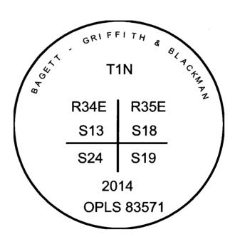
I used a steel tape and magnetic compass in the establishment of the new bearing trees. I used  $16^{\circ}$ East declination, the distances are to a 60d spike in the right hand side of the root crown.
