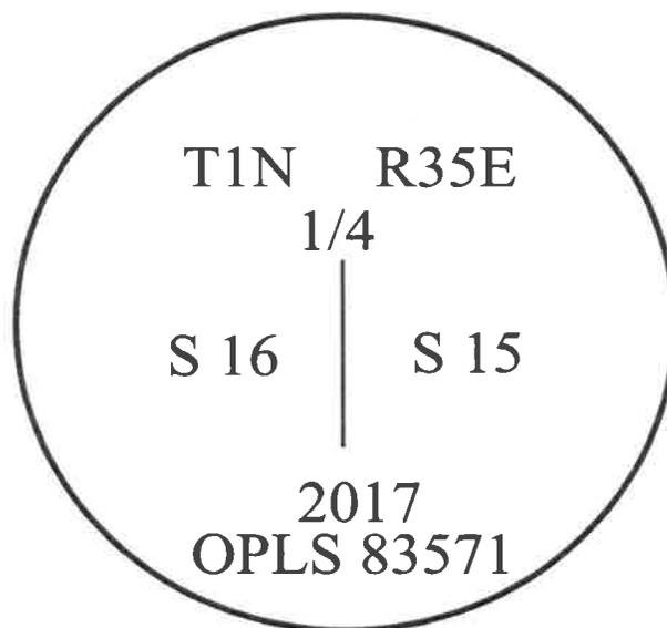
I used a steel tape and magnetic compass in the establishment of the bearing trees. Magnetic declination used was 13° East. Bearings are to a brass washer marked OPLS 83571 in the lower blaze of the tree. Distance is to a spike set in the root crown of the side of the tree.
