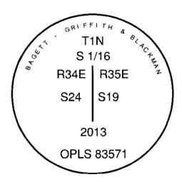
I used a steel tape and magnetic compass in the establishment of the bearing trees. Magnetic declination used was  $16^{\circ}$  East. Bearings are to a washer marked OPLS 83571 in the lower BT blaze.
