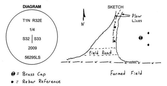
MONUMENT (S) AND ACCESSORIES SET (Procedures and Description) I set a 1 1/2" x 30" galvanized iron pipe with a 2 1/2" brass cap stamped as shown in the diagram above at the proportionate point.
