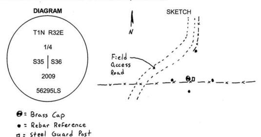
MONUMENT (S) AND ACCESSORIES SET (Procedures and Description) I Set a 1 1/2" x 30" galvanized iron pipe with a 2 1/2" brass cap stamped as shown in the diagram above at the intersection of the east - west fence line and the north - south section line.
