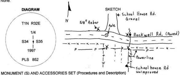
Set a 1 1/4" X 28" car axle with a 3" diameter flange on top at the proportioned point flush with the pavement of Rockwell Road (County Road No. 1064).
