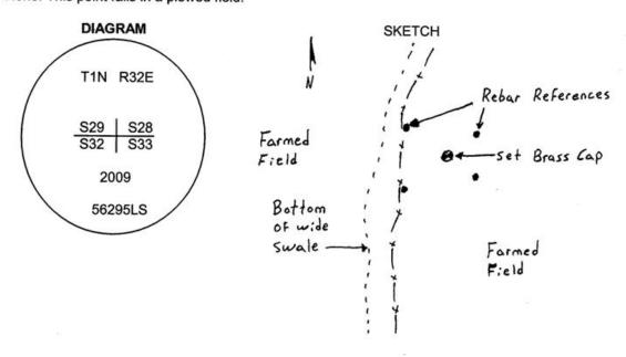
MONUMENT (S) AND ACCESSORIES SET (Procedures and Description) At the proportionate position I set a 1 1/2" x 30" galvanized iron pipe with a 2 1/2" brass cap stamped as shown in the diagram above. The cap is 24" below the surface.
