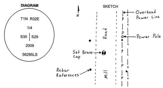
MONUMENT (S) AND ACCESSORIES SET (Procedures and Description) I set a 1 1/2" x 30" galvanized iron pipe with a 2 1/2" brass cap stamped as shown in the diagram above by proportioning the latitude and holding the center of the county road as determined by the right of way fence.
