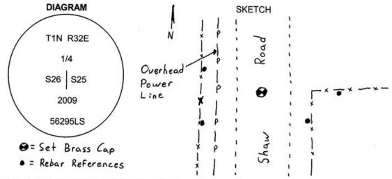
MONUMENT (S) AND ACCESSORIES SET (Procedures and Description) I set a 1 1/2" x 30" galvanized iron pipe with a 2 1/2" brass cap stamped as shown in the diagram above at the position of the nail.
