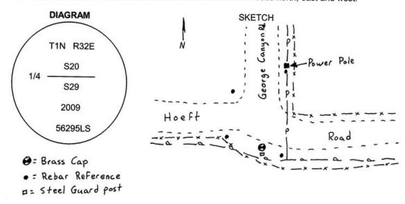
MONUMENT (S) AND ACCESSORIES SET (Procedures and Description) At the proportionate point I set a 1 1/2"x30" galvanized iron pipe with a 2 1/2" brass cap stamped as shown in the diagram above. I set a 6' steel guard post with a monument sign on the south side of the cap.
