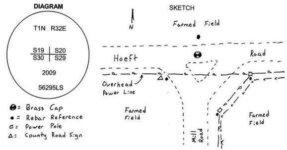
MONUMENT (S) AND ACCESSORIES SET (Procedures and Description) At the intersection of roads running east, west, and south, I set a 1 1/2" x 30" galvanized iron pipe with a 2 1/2" brass cap stamped as shown in the diagram above. The cap is 8 inches below the surface of the road.
