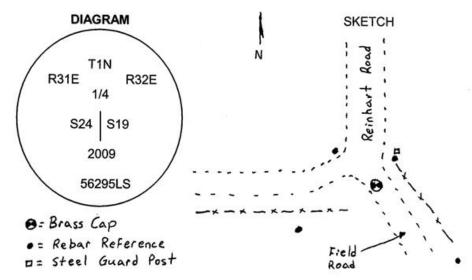
MONUMENT (S) AND ACCESSORIES SET (Procedures and Description) Set a 1 1/2" x 30" galvanized iron Pipe with a 2 1/2" brass cap stamped as shown in the diagram above at the proportioned point. The cap lies 6" below the surface of a farm field access road. I poured concrete around the cap.
