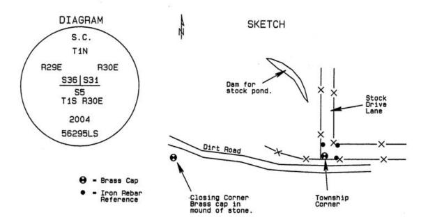
Monument and accessories set: (Procedures and description) I set a 2 3/8" brass cap on a 30" x 1 3/8" O.D. galvanized iron pipe 32" in the ground. The cap was stamped as shown in the diagram above. I attached a County Monument sign to a nearby fence post.
