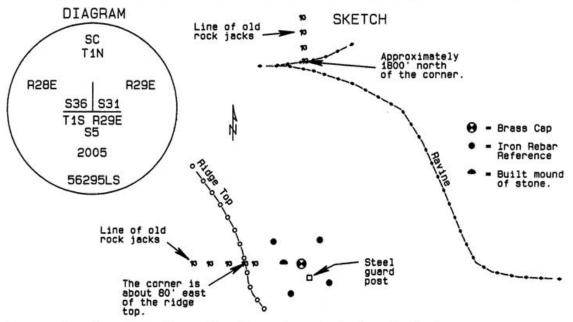
Monument and accessories set: (Procedures and description) At the position of the decayed post I set a 2 3/8" brass cap on a 1 1/2" x 30" galvanized iron pipe 30" in the ground with an 18" collar of stone. I built a mound of stone with a 4' base by 2' high, 4 feet west of the cap. I set a 6' steel guard post along side with a county monument sign attached. I buried the stone along side.
