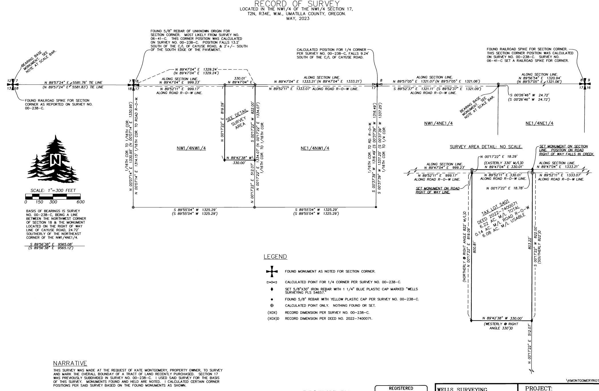
THIS SURVEY WAS MADE WITH A ONE PERSON CREW USING A LECIA GS14 GPS RECEIVER OPERATED OVER THE OREGON REALTIME GNSS NETWORK. CONTROLLING TIES AND SET MONUMENTS WERE VERIFIED BY MULTIPLE OBSERVATIONS.
