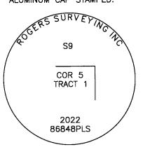
SET FLUSH IN GROUND IN CENTERLINE OF DRAINAGE DITCH AT WEST EDGE OF GRAVEL.
