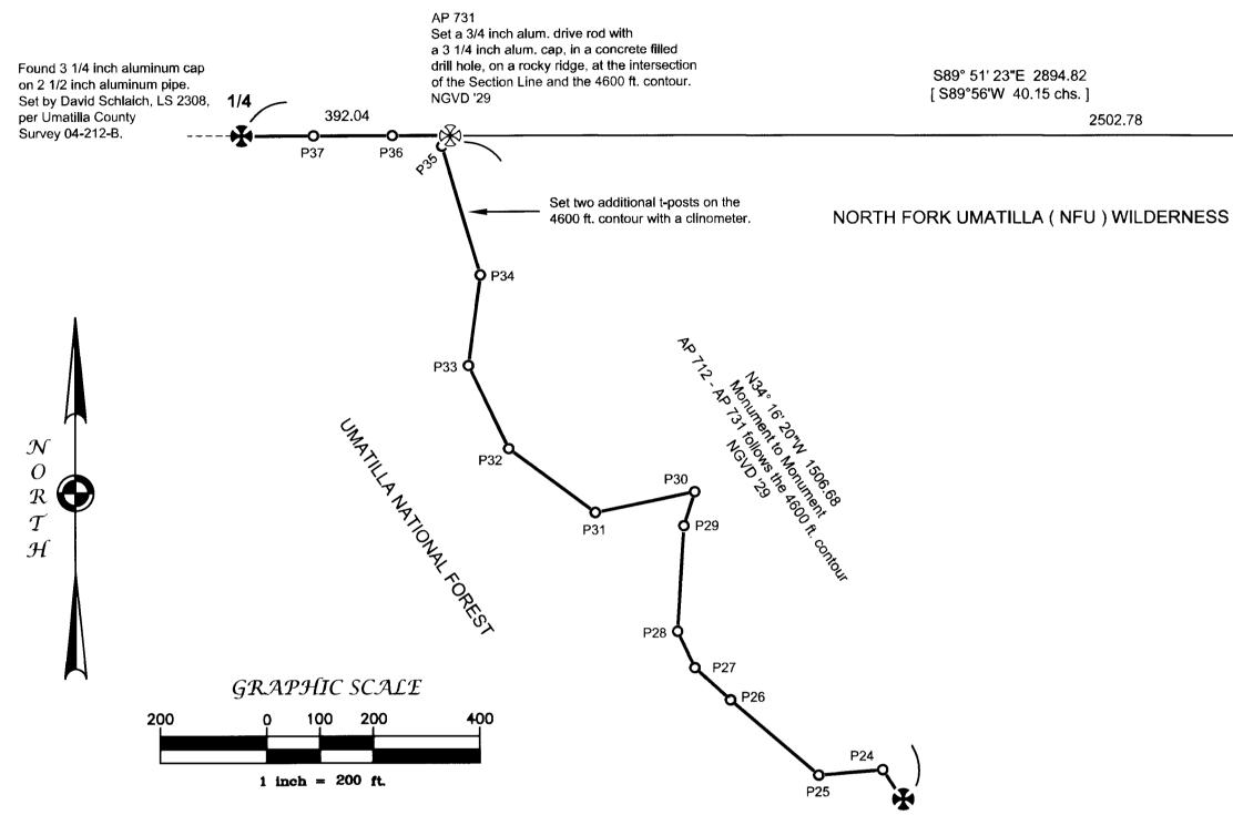
Latitude & Longitude for Points on Line and Angle Points (NAD '83) Point or AP# Longitude Description Latitude NGVD '29 W118°04'58.807" 3 1/4" alum. cap on 2 1/2" alum. pipe 6-foot steel t-post with WB sign attached N45°42'51.0" W118°04'59.3" 32" Douglas fir line tree with WB sign attached P25 N45°42'50.9" W118°05'01.0" N45°42'52.3" W118°05'03.4" 6-foot steel t-post with WB sign attached P26
