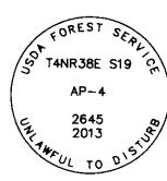
SET A 5/8" X 30" REBAR WITH A 3 1/4" ALUMINUM CAP MARKED AS SHOWN
