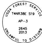
SET A 5/8" X 30" REBAR WITH A 3 1/4" ALUMINUM CAP MARKED AS SHOWN
