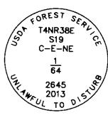
SET 3  $\frac{1}{4}$ " ALUMINUM CAP ON 3"X36" ALUMINUM PIPE MARKED AS SHOWN
