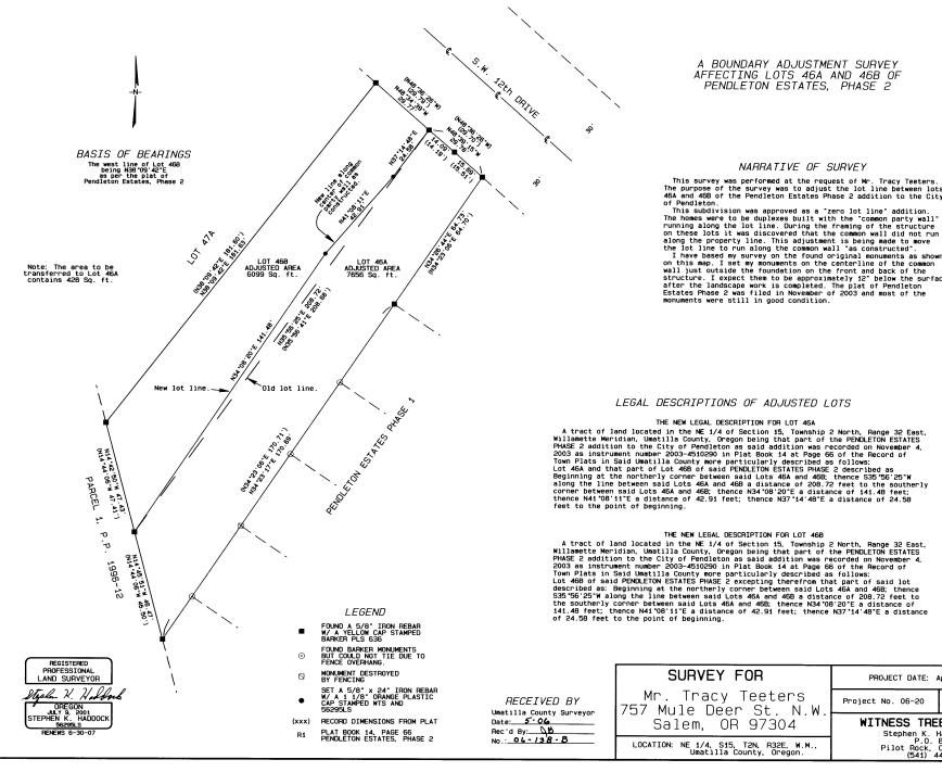
The purpose of the survey was to adjust the lot line between lots 46A and 46B of the Pendleton Estates Phase 2 addition to the City
