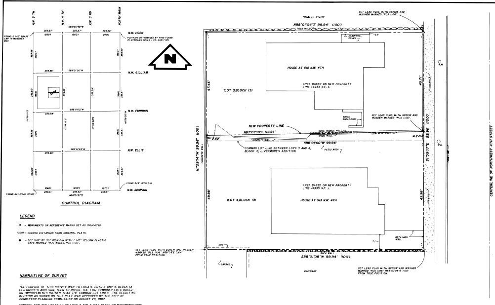
CONTROL FOR THE LOCATION OF LOTS 3 AND 4 WAS BASED ON MONUMENTATION FOUND AS SHOWN ON THE CONTROL DIAGRAM. THE SURVEY WAS MADE WITH T-16 THEODOLITE, STEEL TAPE, AND INFFAR RED DISTANCE MEASURING EQUIPMENT. BEARINGS ARE BASED ON MONUMENTS ON N.W. 5 TH STREET AS INDICATED ON THE CONTROL DIAGRAM.
