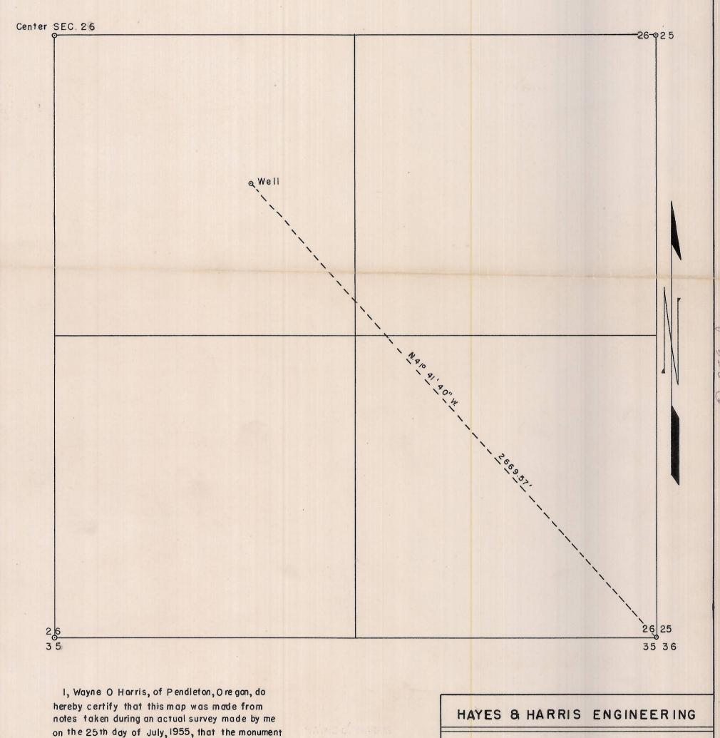
hereby certify that this map was made from notes taken during an actual survey made by me on the 25th day of July, 1955, that the monument shown on this map, consisting of the intersection of old fence lines, is the S.E. corner of Sec. 26, T. 4N, R. 34E.W.M., which is verified by the testimony of local residents.
