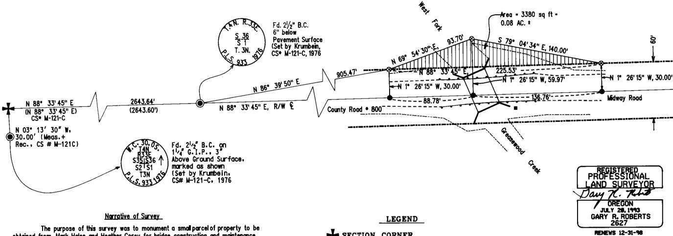
obtained from Mark Hales and Heather Corey for bridge construction and maintenance. The northeast wingwall of the bridge was inadvertently built outside of the right-of-way of County Road \*800. Midway Road due to the fact that the section line lies near the middle of the south travellane in the vicinity of the bridge and our bridge crew was not aware of it.
