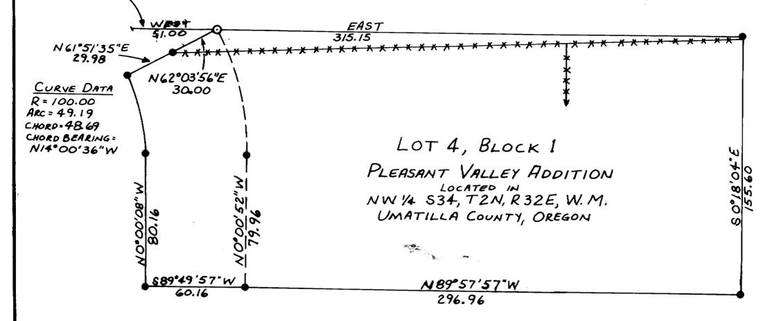
BEARINGS ARE BASED ON THE RECORD BEARING OF THE LINE FROM THE SOUTH EAST TO THE SOUTH WEST CORNERS OF LOT 4 AS SHOWN ON UMATILLA COUNTY SURVEYOR'S PLAT NO, P-108-B FILED JUNE 1978.
